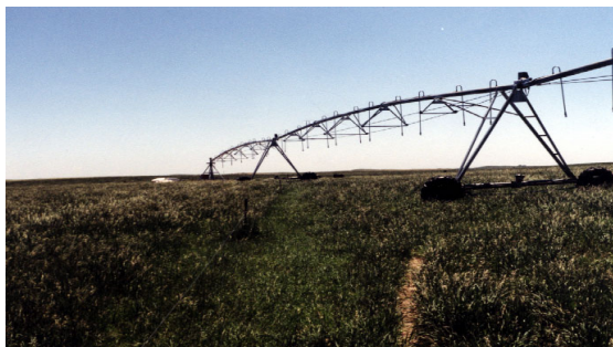
Electric Fence, single wire, partitions paddocks on center pivot of cool season grass mix. Notice that petition fence is “off center” or not on the radius of the circle. This allows the irrigation system to “walk” over the fence one tower at a time.
