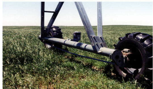
Sprinkler tower equipped to run over electric petition fence. Note pipe that has been bolted onto the frame. This prevents fence wire from becoming entangled in running gear.
